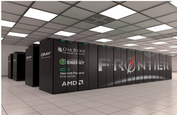
Figure: The fastest supercomputer in the world: Frontier, HPE CRAY EX235A, AMD OPTIMIZED 3RD GENERATION EPYC 64C 2GHZ – USA, Oak Ridge – Rmax = 1.5 Exa Flops = 1.5 \times 10^{18} Flops, using 21'000kWh – foto: Oak Ridge
